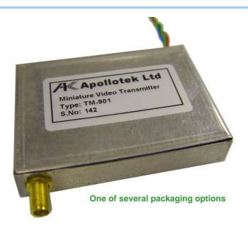
The TM-901 is a small size, low weight, high efficiency transmitter optimised for L-Band, Upper L-Band and S-Band Video and Telemetry data transmission applications requiring RF Power outputs up to 1 Watt.
