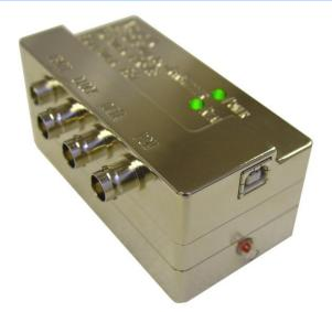
The Apollotek Model APK8768-B combines the features of the Apollotek APK8764 USB PCM Simulator with a low power RF Transmitter module and a rechargeable battery pack. This PCM Simulator unit is set up and powered through a USB Port connection to a host PC and it provides a high performance programmable PCM Simulator with programmable low power transmitter centre frequency to provide a portable radio telemetry link and groundstation test capability.
