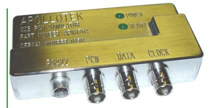
The Apollotek Model APK8764 is a general purpose PCM Simulator which is set up through a USB connection to a host PC. The unit is also powered through the USB Port. The Model 8764 is designed to work directly with the Apollotek GDSmate Telemetry Environment Software package to provide a high performance programmable PCM Simulator.
